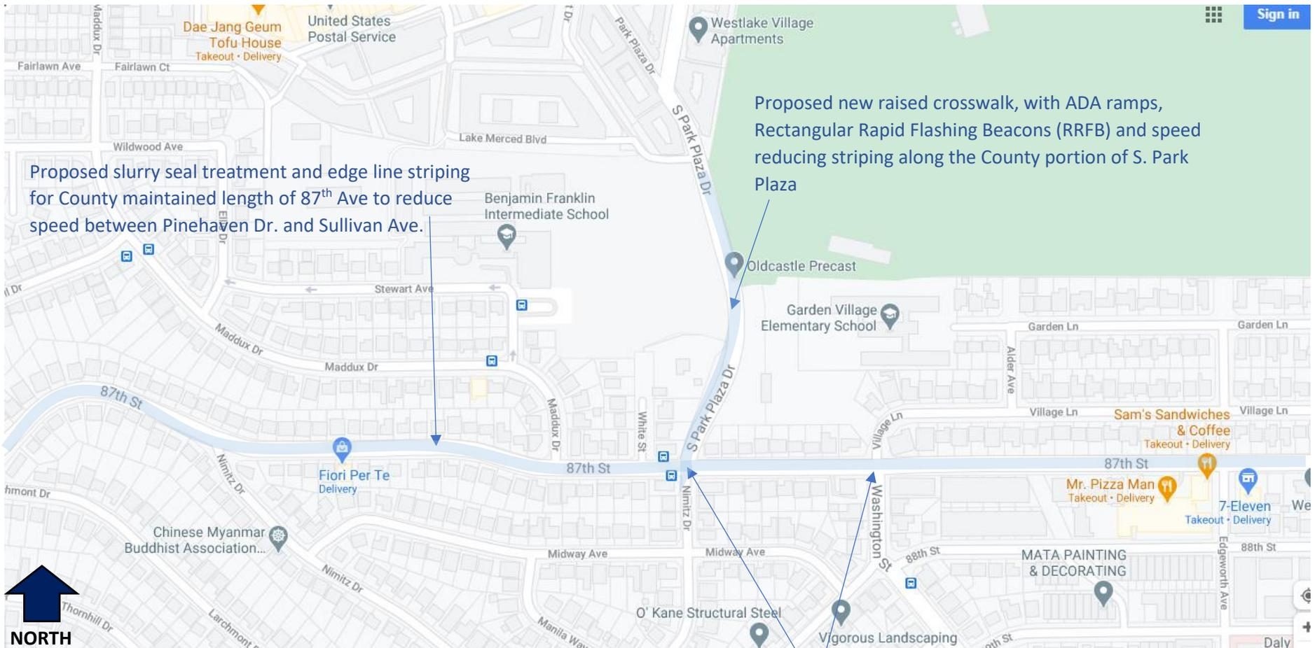
Proposed slurry seal treatment and edge line striping for County maintained length of 87<sup>th</sup> Ave to reduce speed between Pinehaven Dr. and Sullivan Ave.
