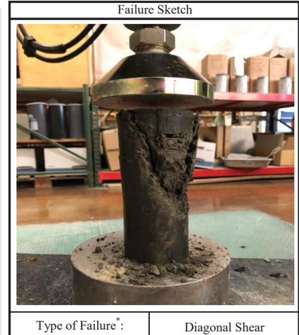
\*Bulge, Diagonal Shear, or Longitudinal Splitting
