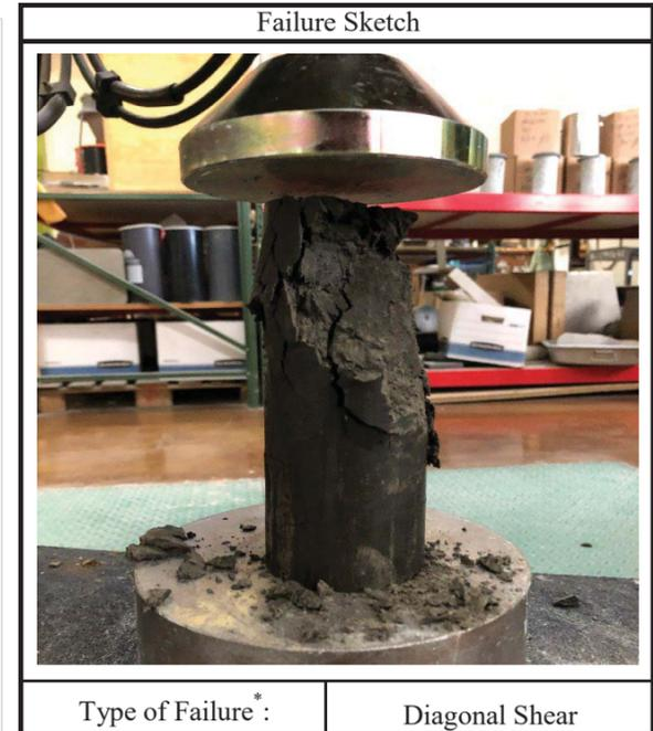
\*Bulge, Diagonal Shear, or Longitudinal Splitting
