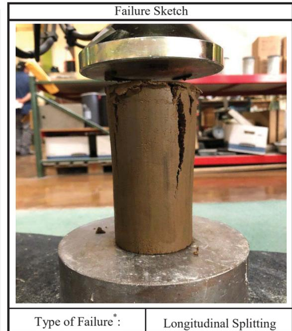
\*Bulge, Diagonal Shear, or Longitudinal Splitting
