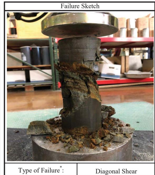
\*Bulge, Diagonal Shear, or Longitudinal Splitting
