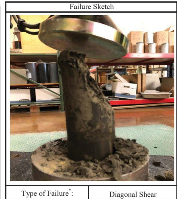
\*Bulge, Diagonal Shear, or Longitudinal Splitting
