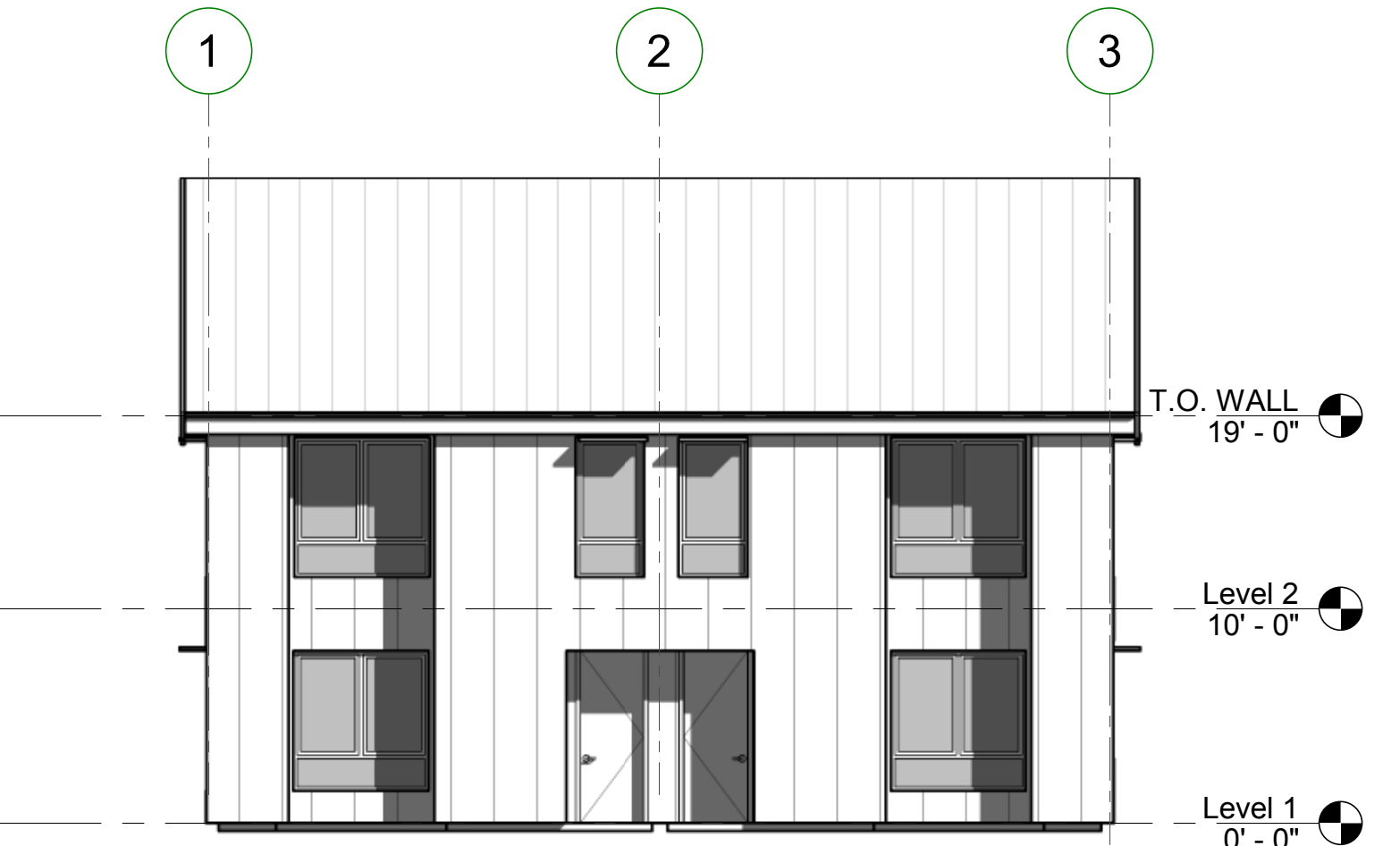
BLDG TYPE A - SOUTH ELEVATION 5 1/8" = 1'-0"
