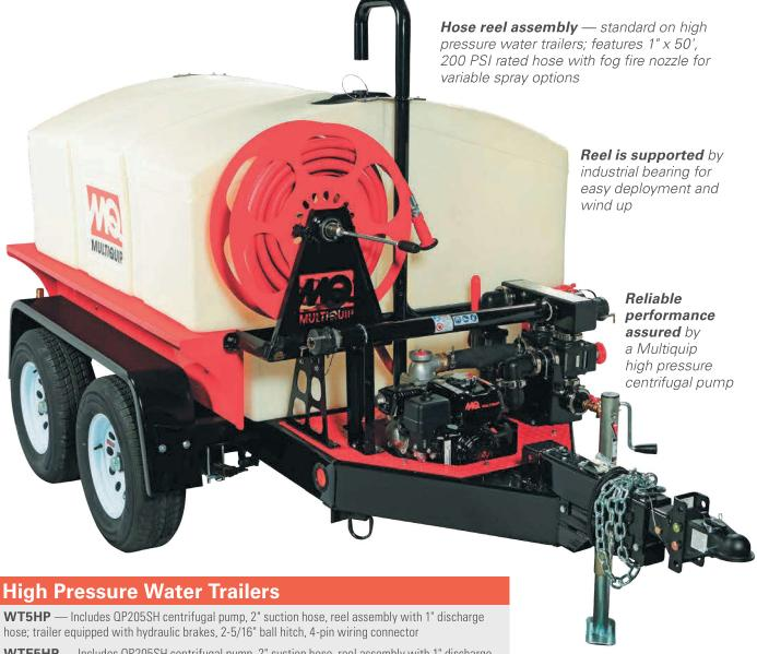
**WTE5HP** — Includes QP205SH centrifugal pump, 2" suction hose, reel assembly with 1" discharge hose; trailer equipped with electric brakes, 2-5/16" ball hitch, 7-pin wiring connector
