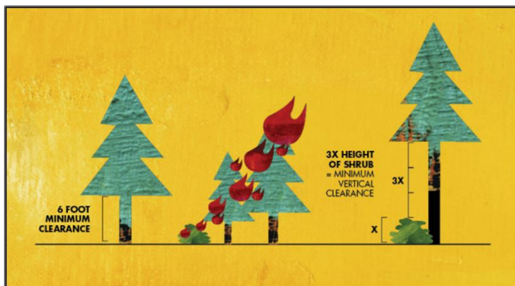
Figure 1: Ladder fuel clearance guidelines
