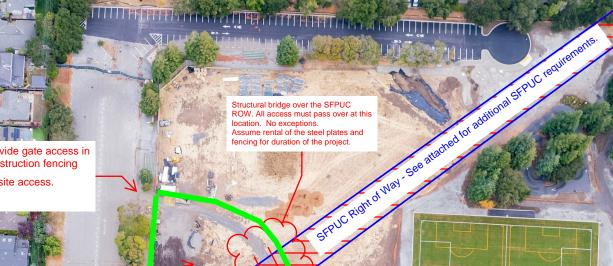
Structural bridge over the SFPUC ROW. All access must pass over at this location. No exceptions. Assume rental of the steel plates and fencing for duration of the project.
