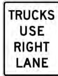
Figure 8: Trucks Use Right Lane Signage (R4-5)
