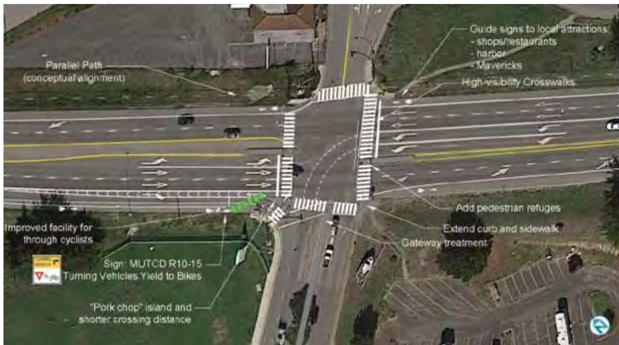
Figure 10: Highway 1 and Capistrano Road (S) Conceptual Improvements
