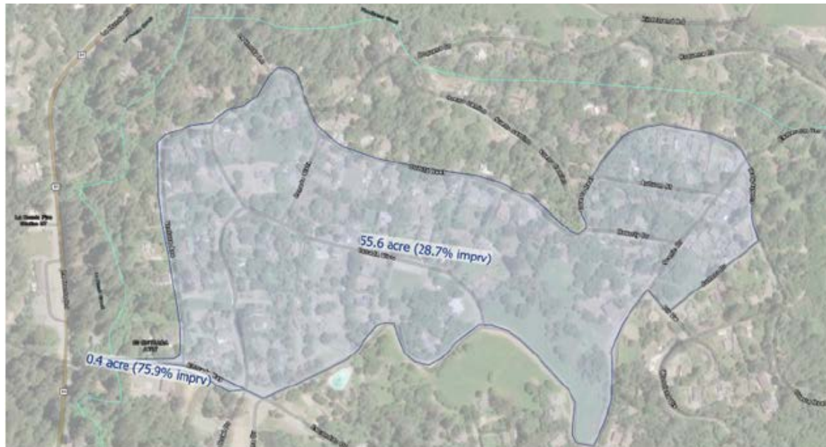
Figure 7. Drainage Areas for Entrada Way Roadside Drainage System at East Side of Creek Culvert.
