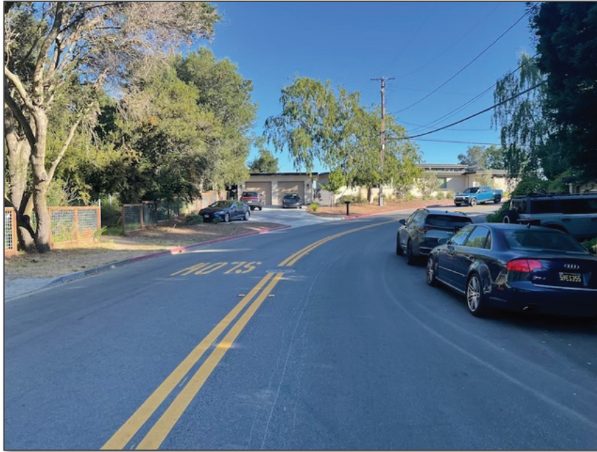
Photo taken from approximate location of a car turning left into the existing fire road proposed to be a new entrance and parking lot. Approximately 170 feet of Stopping Sight Distance
