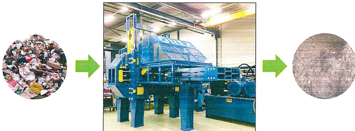
Anaergia Orex Press Detail (showing infeed and output)
