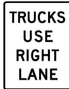
Figure 8: Trucks Use Right Lane Signage (R4-5)
