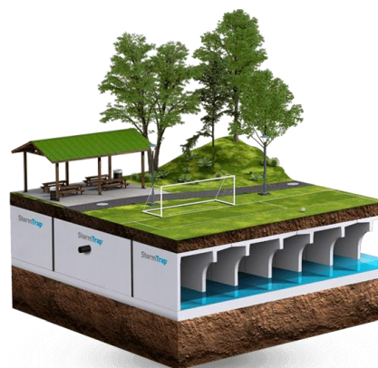
Figure 1.15. Subsurface storage system, generic example.
